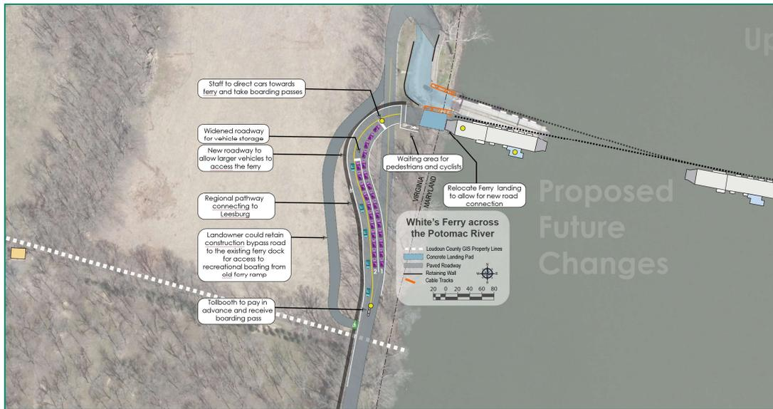
Figure 4-10: CAD drawing of Proposed Roadway Adjustments on Virginia Side
