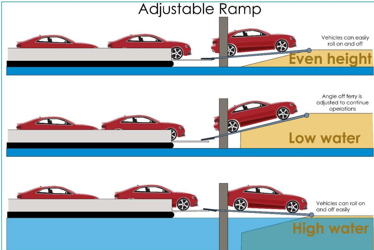
Some ferry slips use a hinged steel plate ramp like those of the Toronto Island ferry system, which connects an island chain with downtown Toronto, Ontario (see Figure 4-16 and Figure 4-17). This type of ramp can be raised or lowered to match tidal movements.
