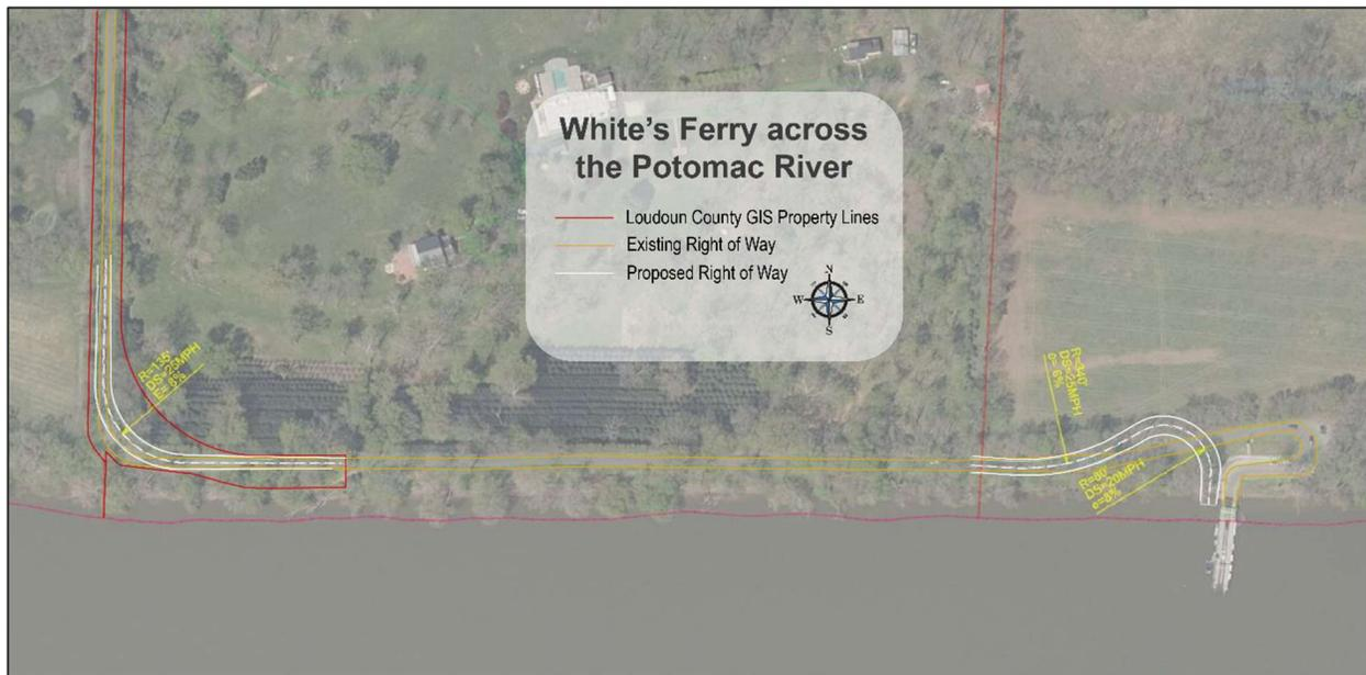
A second component of infrastructure improvements should include geometric improvements to the 90 degree turn on Whites Ferry Road south of the Ferry terminal to increase the turn radius as much as possible while remaining within the existing right- of-way (see Figure 4-11).
